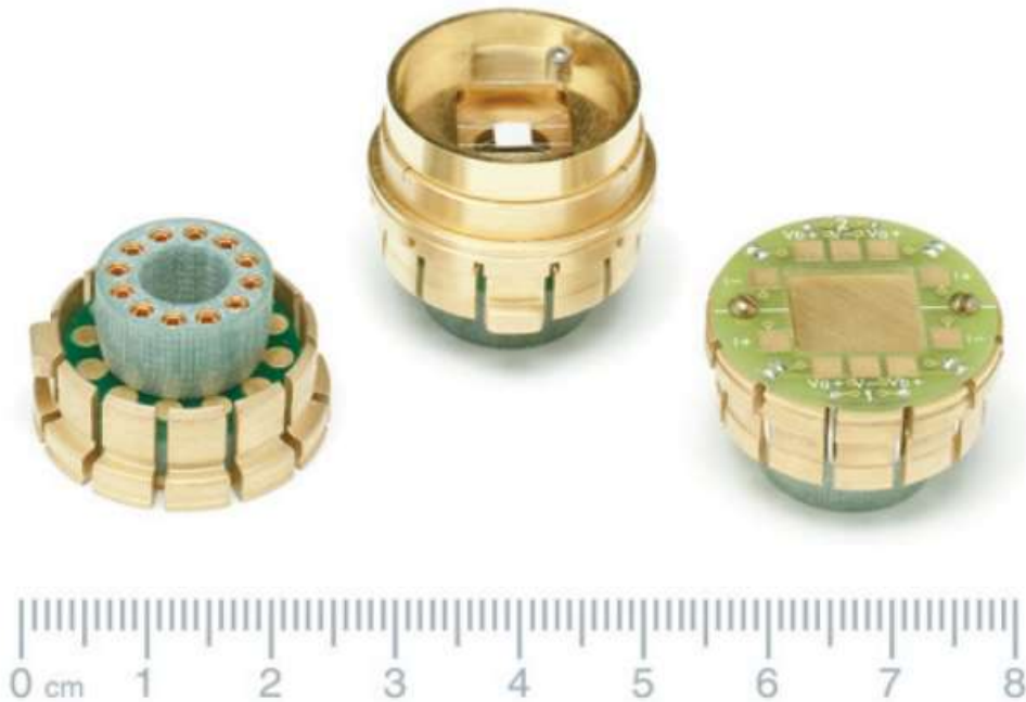
Figure 1.2 — Image of a standard calorimeter cell of the Heat Capacity option Heat Capacity .
